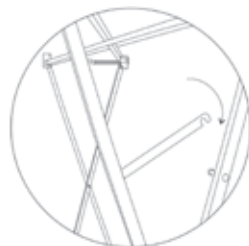
Fix up the plastic connector clip the steel strip and the ricet
