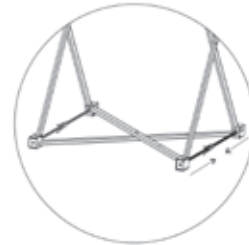
Fix up the plastic connector clip the steel strip and the ricet
